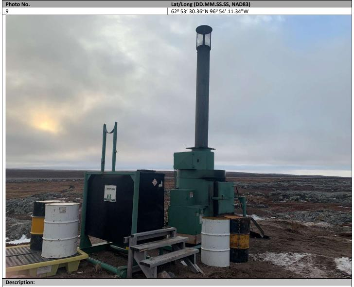
Incinerator used to dispose of combustible garbage.
